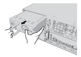
Figure 2. Removing the Power Supply
